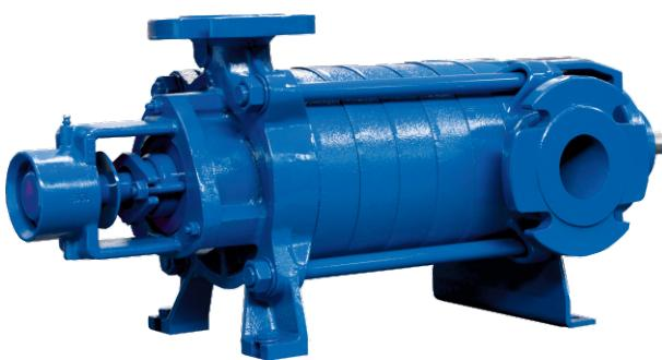
**USE:** TS pumps are suitable for clean or slightly dirty liquids and are used for boilers feeding, fire fighting plants, autoclaves, water supply systems, washing plants, irrigation, to pump hydrocarbons and whenever high pressures are required.
