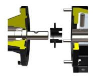
Connection to the motor drive system is through a coupling flange and pin coupled to the shaft. This system is the most economical, versatile and reliable, as it minimizes manufacturing costs and times. The pin on the shaft has the added advantage of presenting the same resistance qualities in both rotating directions yet without reducing the space available for the seal system.
