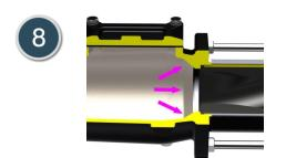
The inlet stator area is conical in shape with a large cross section. This, together with the compactness of the joint enables easy passage of the product, the NPSHr, and feed of products with large solids into the pumping part.
