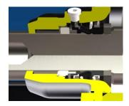
Standard construction with bi-directional single mechanical seal. The space between the shaft seal and the lantern is designed to house various types of seals such as single mechanical seals with quench, back-to-back or tandem double seals, gland packing systems with or without flushing.
