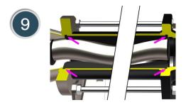
The two sides of the stator are fitted with integrated seal systems which avoid the use of additional O rings, and also prevent the body and flange from rotating if the rotor and stator jam during pump start up.
