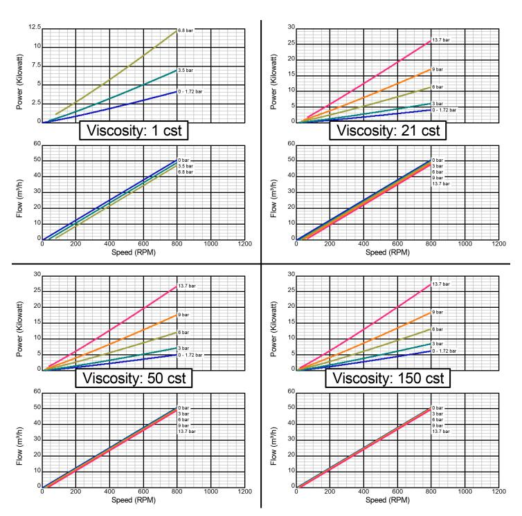
There are many additional factors to consider when selecting a pump, including (but not limited to) suction conditions, temperature limitations and material compatabilities. Curve data is typical only, octual performance may vary. Consult the factory or an authorized Tuthill Pump Group representative for assistance.
