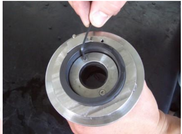
15) The use of the extractor to pull out the bushing from the casing is recommended.
