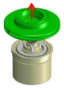
8) Check impeller thrust bearings; replace it in case of damage or wear.
