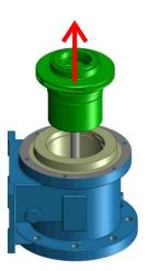
6) Extract the internal cartridge (RWP) from the pump.
