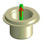
10) Check shaft status, replace it in case of damage or wear
