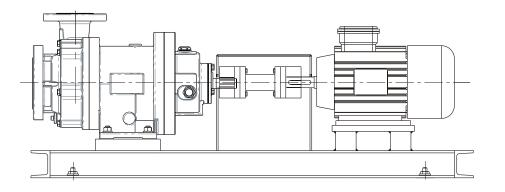
Fit the two elastic coupling halves on the pump and on the motor.
