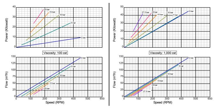
There are many additional factors to consider when selecting a pump, including (but not limited to) suction conditions, temperature limitations and material compatabilities. Curve data is typical only, actual performance may vary. Consult the factory or an authorized Tuthill Pump Group representative for assistance.
