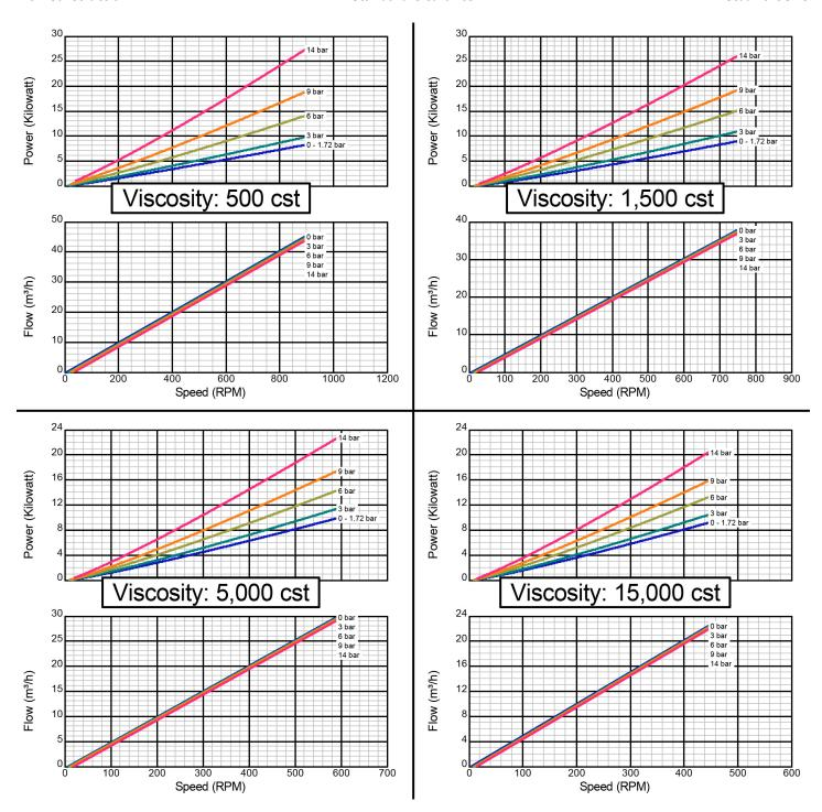
Iron Construction Standard Clearance 2" Std. Port Size
